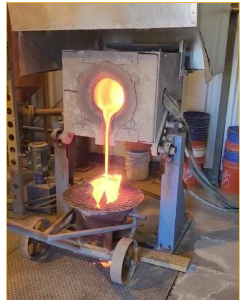
Induction melting furnace
